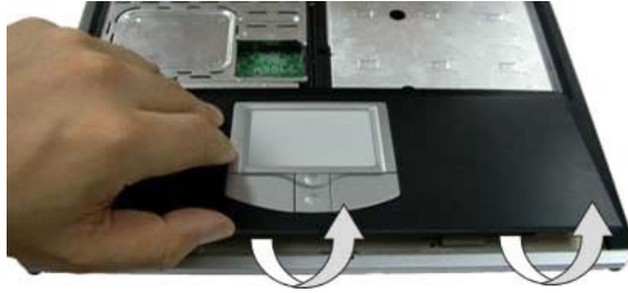
Fig. 10 Flipping over the touchpad assembly
